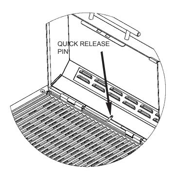
With the quick release pin removed, grasp the lid, lifting on the left side to clear the hinge and slide it to the left until clear of the hinge pin on the right. Once the lid is removed, it can be washed in warm, soapy water.
