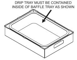
To prevent the contents of the drip tray from smoking, place 1 cup of water (or enough to cover the bottom of the pan) in the drip tray before cooking. The replacement for the disposable drip tray is Kenyon part #B96001.
